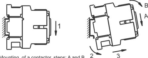
Mounting, of a contactor, steps: A and B.
