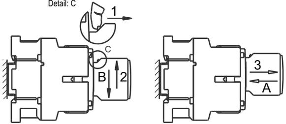
Mounting, of an auxiliary block, steps: A and B.
