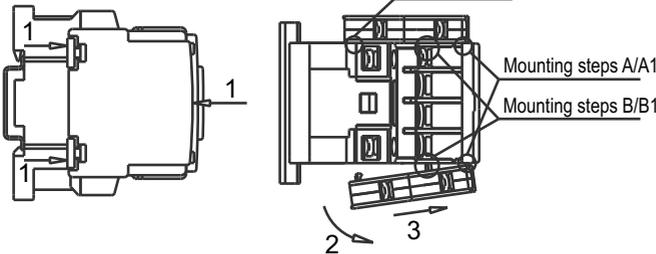
Mounting, of an auxiliary block, steps:
