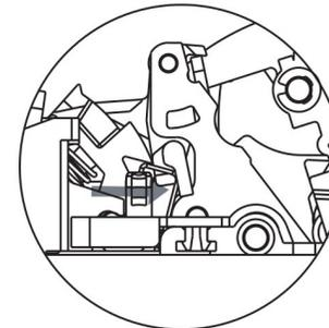
You need to gently push the right slot into the closing direction before installation.
