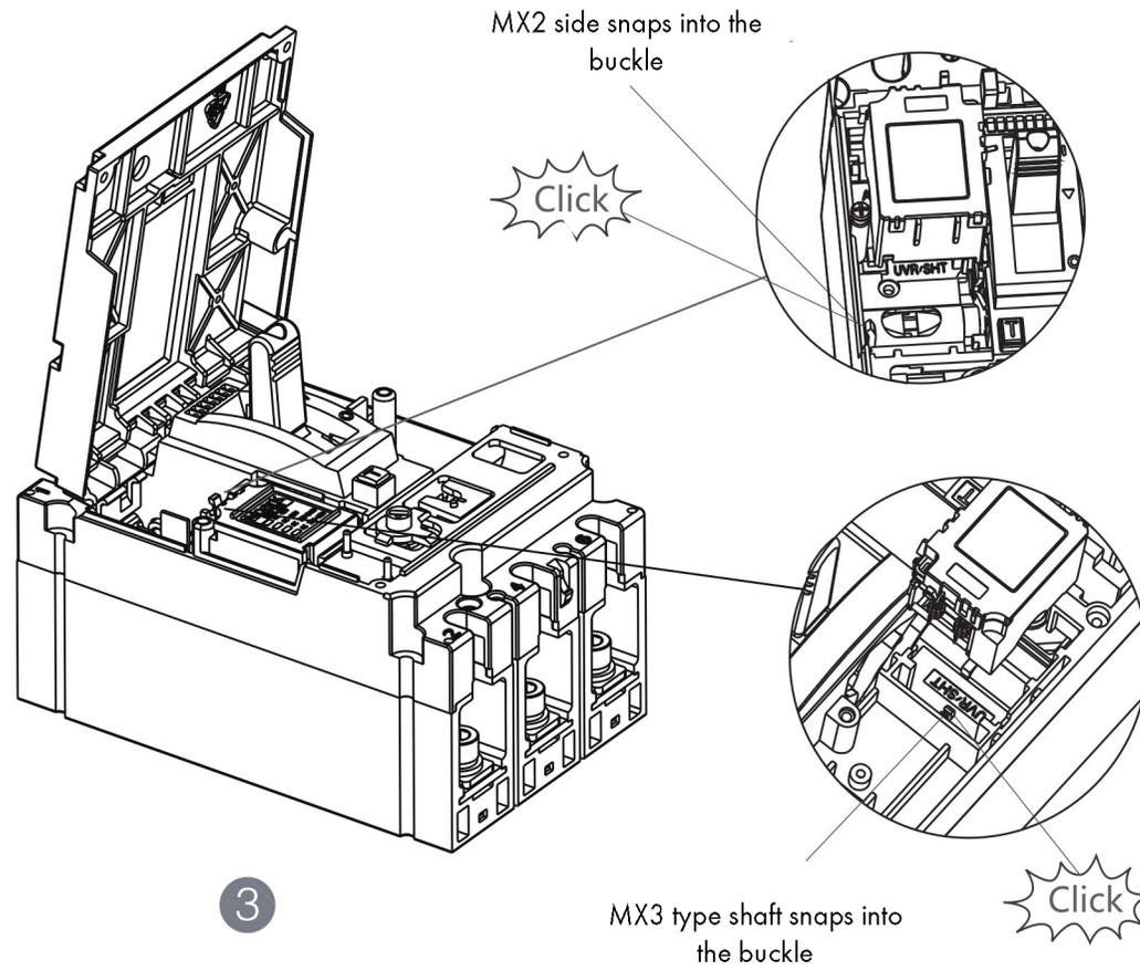
When installing MX2 moulded case circuit breaker, you need to push the handle gently in the closing direction.
