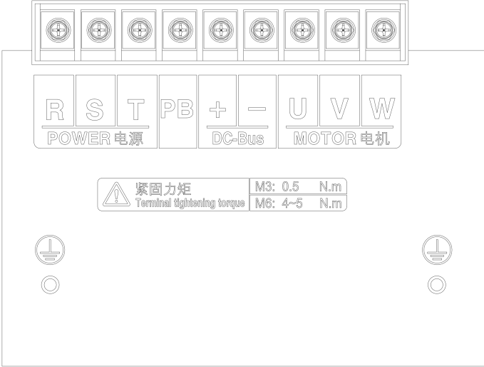
d) Schematic Diagram of Terminals (EM730-030-3/3B~EM730-037-3/3B)
